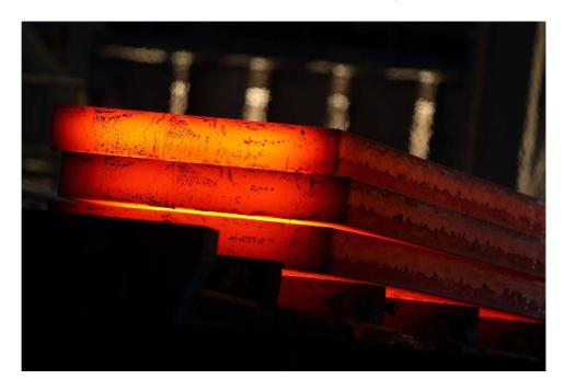
These semi-finished products are the basis for manufacturing hot-rolled products at the upgraded 1700 mill. Besides, new slabs are in high demand among the re-rollers due to improved chemical composition and excellent geometric characteristics. Steel products manufactured from such semi-finished products can be used in all applications; especially, they are in demand in the
