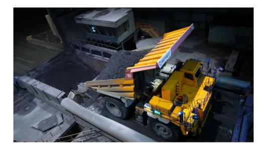
From the open-pit mine, ore and rock are transported by trucks to the crushers. Once crushed, they are transferred to the conveyor system to travel 2.3 kilometres in 16 minutes. After arriving to the surface of the mine, ore and rock are loaded into railway cars. Ore is then delivered to the crushing plant, while rock is transported to the dump area.
