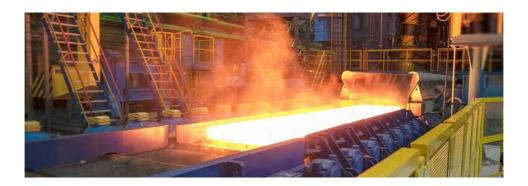
A large-scale revamp of 1700 HSM began in 2017 and had several phases. In the first phase, reheat furnace No. 1 was commissioned and a heavy-duty coiler was installed. In the second phase, an intermediate coiler (coilbox) was installed along with hydraulic descalers, a reversing roughing mill, and other process equipment. The finishing mill stands were also reinforced and modernized.
