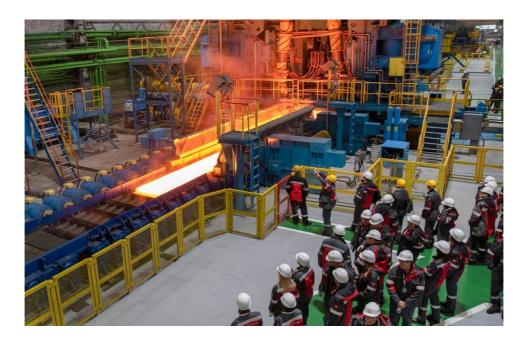
The new reversing mill with equipment for vertical breakdown of slabs is equipped with an automated control system, which allows to produce quality feedstock for the finishing mill. The coilbox installed after the roughing mill provides for intermediate coiling of long workpieces during the production of heavy coils.
