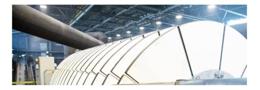
The new equipment allows reducing the cost of iron ore processing. The operation of the filters is supported by a stand-alone unit with the pump, which ensures energy savings of 640 kWh vs. the dismantled DOO-100 fabric filters. KDF-90 can be supplied with a thicker mass for drying, which reduces the consumption of process water. Ceramic consumables require replacement every year and a half, while fabric replacement was required every month.
