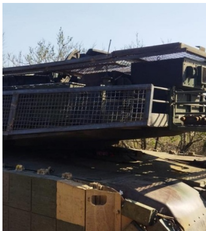
Steel anti-drone screens for different types of equipment increase survivability under intense combat
