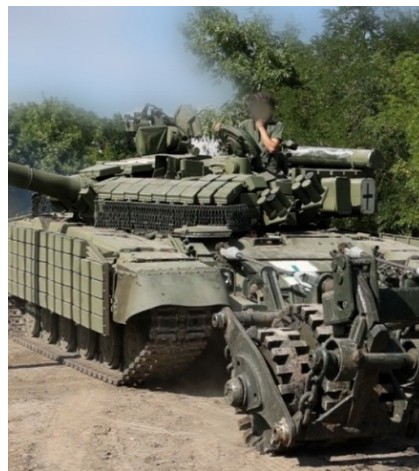
Mine trawls help tanks safely clear minefield
