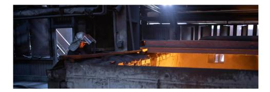
Wearing a heat-protective coat with hood and a visor, Serhiy peered down into a glowing orange stream of searing liquid metal at Ukraine's Zaporizhstal steel plant. The blast furnace worker was as usual testing a stream of molten crude iron at around 1,400 degrees centigrade (2,552 Fahrenheit) for impurities. And yet just 40 kilometres away, some of the fiercest fightings of Russia's invasion times are playing out as a part of Ukraine's counteroffensive.
