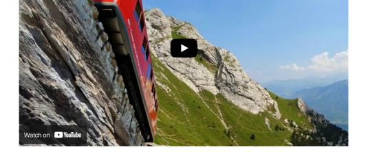
The rack railway is another rail wonder. In general, it is laid in the mountains so that trains can manage routes with a large changes in altitude. To do this, an additional rack rail is laid between a pair of conventional rails. A special gear is installed on the bottom of the train and it clings to this rail and allows the train to safely overcome sharp ups and downs. This type of transport is most popular in the
