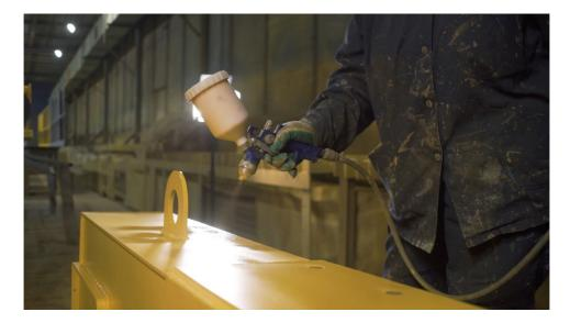
Only properly prepared products and structures should be painted. After all, in the case of steel, paint is not only a decorative element; it is part of the comprehensive protection against corrosion and premature failure.
