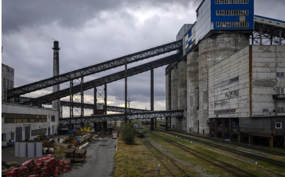
Conveyor belts carry coking coal to storage silos at Metinvest BV's Pokrovske mine near Pokrovsk, Ukraine on Friday Oct. 25, 2024. Photographer: Christopher Oechicione/Bloomberg
