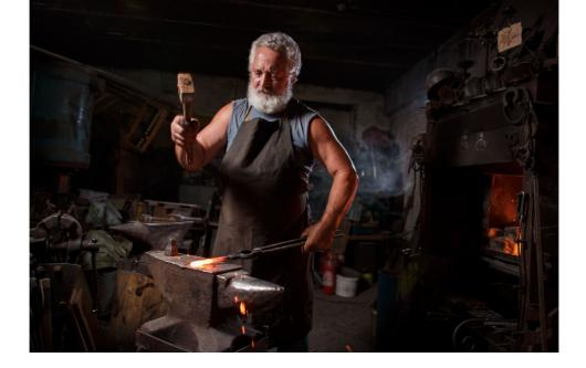
For example, a cherry-coloured shade signals a melting temperature for the steel of 800°C, dark yellow signals over 1,000°C, and bright white indicates 1,250°C.
