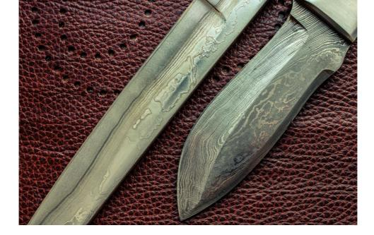
Damascus steel was made differently from others, being based on high-carbon steel. It was practically cast iron that retained its forgeability. While it was molten, pieces of low-carbon metal were added, which, when cooled, gave the weapon excellent cutting properties.
