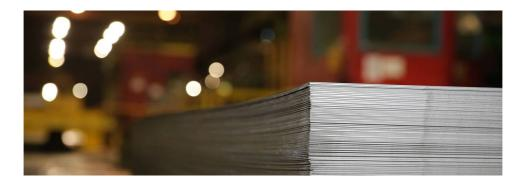
Boron steel is used to manufacture parts for agricultural and industrial machines: grader blades, caterpillar tracks, crushers, knives and saw blades, ploughs and discs for harrows, among others. For the machines to work longer without breaking down, such parts must have high strength, as well as shock and wear resistance.
