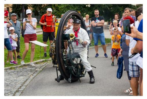
At first glance, the **Dynasphere – a steel wheel** about three metres in diameter – seems to be another steampunk installation. However, it is a real monowheel vehicle, a design that was patented by Dr John Archibald Purves from the UK in 1930. The inventor's idea for the monowheel was inspired by Leonardo da Vinci sketches.
